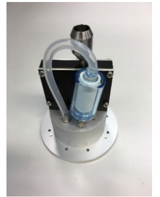
Optical Particulate Counter
