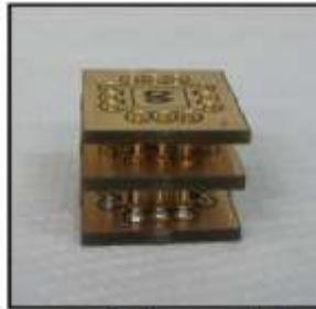
The sensor is the central part. It is equipped with two **protection parts** (on the top and on the bottom) during its handling and storage.
